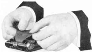
Fig. III. Threading Red Paper into Reel.
