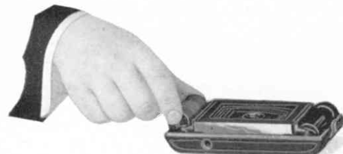
Fig. II. Inserting the Film.
