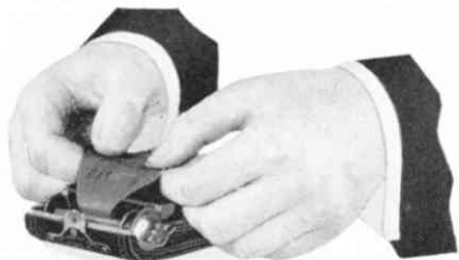
Fig. III. Threading Red Paper into Reel.
