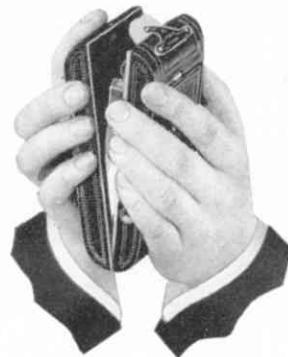
Fig. I. Removing the Back.
