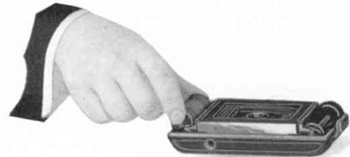
Fig. II. Inserting the Film.
