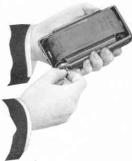
Fig. IV. Binding the Red Paper on Reel.
