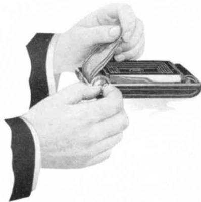
Fig. I. Holding the Red Paper Taut while Turning Key.
