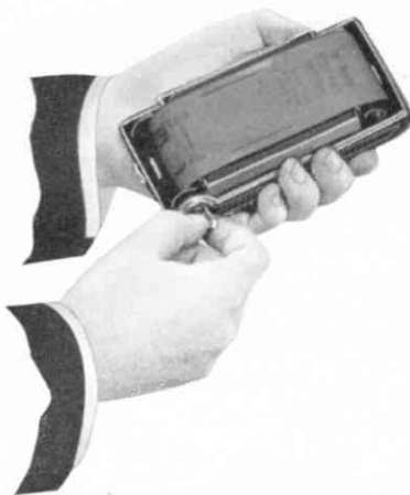
Fig. IV. Binding the Red Paper on Reel.
